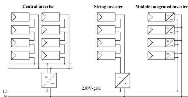
Figure 1: Concepts for the grid connection of solar plants [2]
