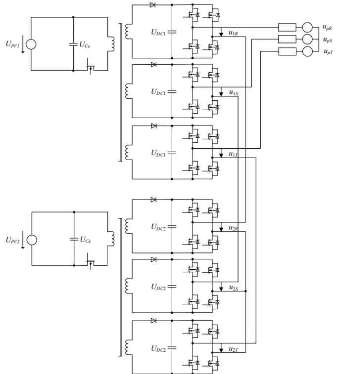
Figure 3: Layout of the implemented photovoltaic multilevel-inverter
