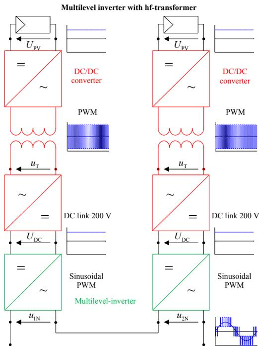
Figure 2: Principle Topology of the photovoltaic multilevel-inverter [2]
