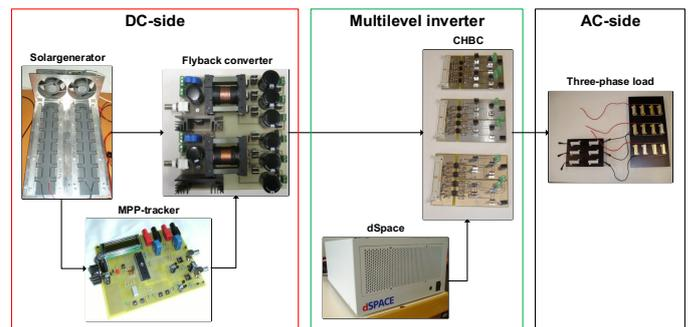
Figure 5: Prototype of the module integrated photovoltaic multilevel inverter
