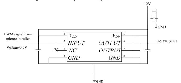
Figure 11: New amplifier circuit with MOSFET driver
