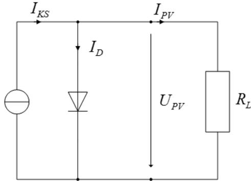
Figure 6: One diode representation of solar module [1]
