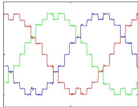
Figure 4: Measured eleven-level output voltage waveform [1]
