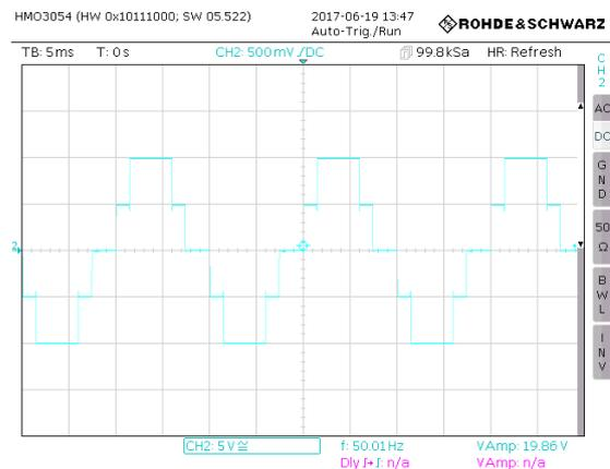
Figure 12: Measured 5-level output voltage
