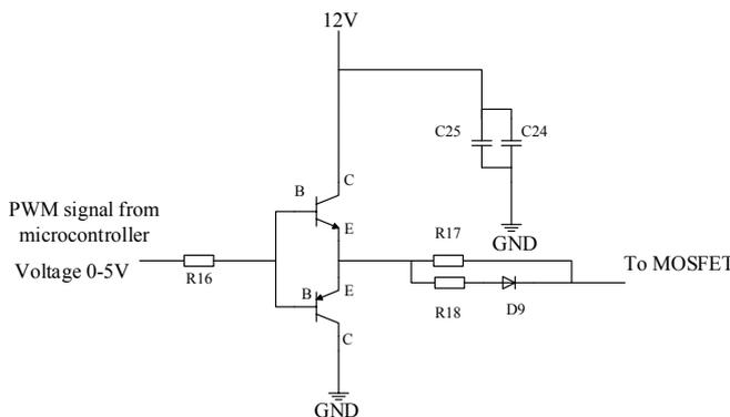
Figure 9: Originally implemented amplifier circuit
