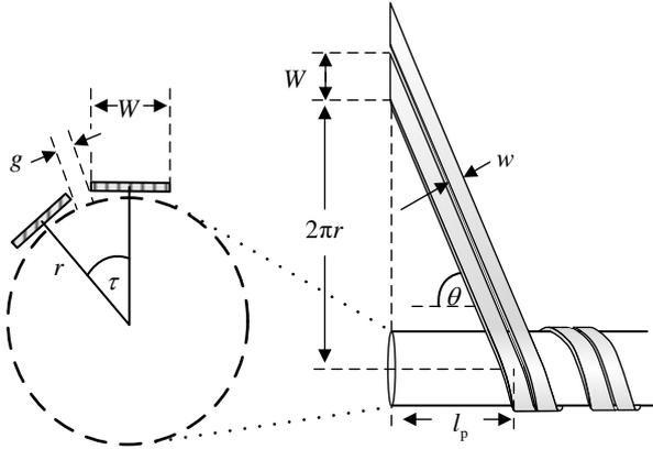
Figure 1. Cross section and side view of a HTS layer [10]
