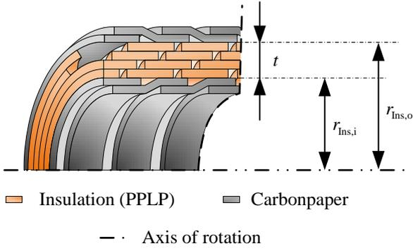
Figure 2. Polypropylene laminated paper insulation [14]
