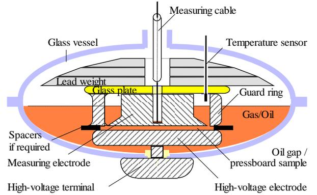
Figure 2. Test cell for determination of the electrical conductivity [4]
