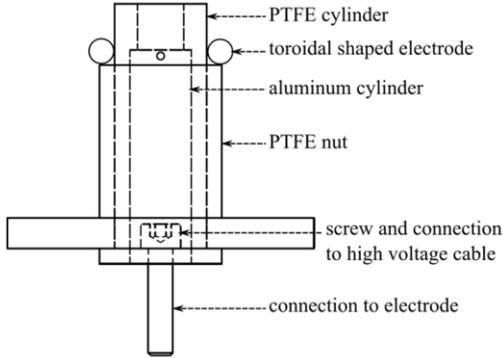
Figure 1. Scheme of the PTFE cylinder for high voltage connection
